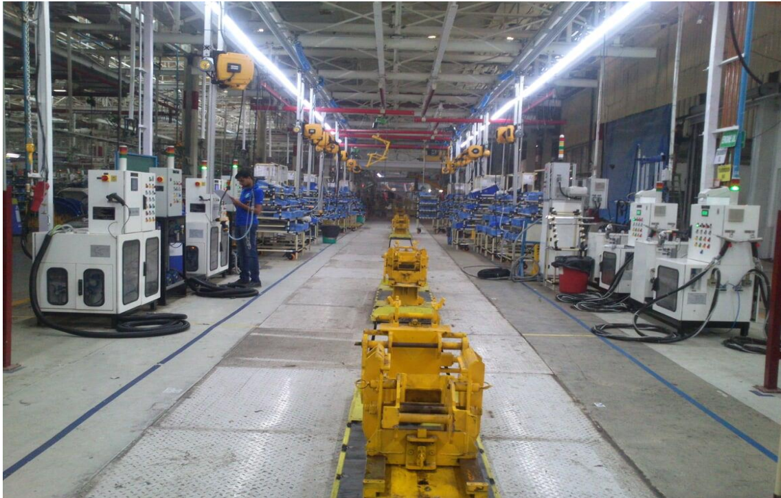
Fig. Automated Liquid Dispensing Systems with common server data integration
