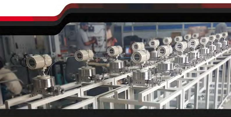
Fluidyne Oscillating Piston flowmeter series is the industry standard for flow measurement of liquids. Virtually unaffected by variations in density of the product, makes it one of the best instruments for Chemical Processing, Life Sciences, Food and Beverage and Hydrocarbon process industries.
